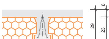
strop Porotherm 23/50/6 strop Porotherm 23/62.5/6
