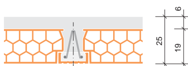
strop Porotherm 19/50/6 strop Porotherm 19/62.5/6
